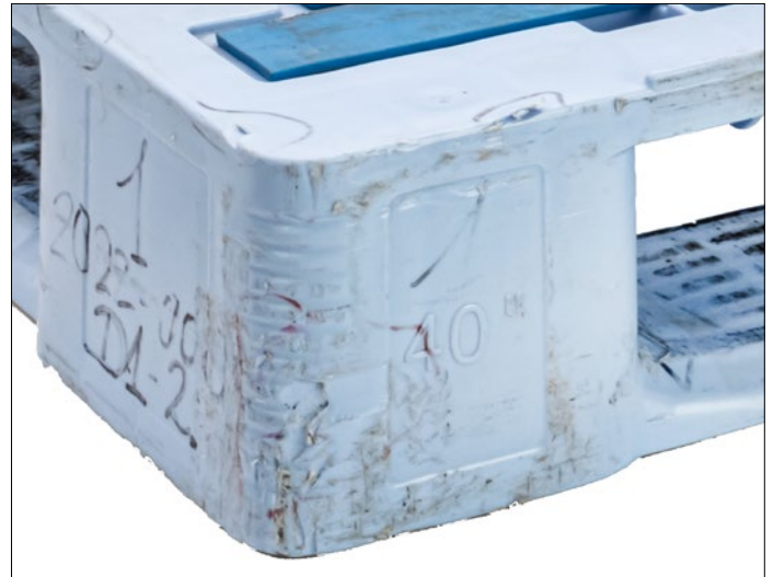
The pallet feet are free from cracks, hairline cracks or other damages.
